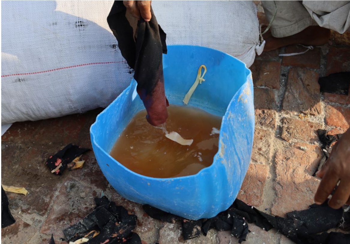
A worker dipping a piece of textile in bleaching chemicals to test if the material is fit for bleaching
